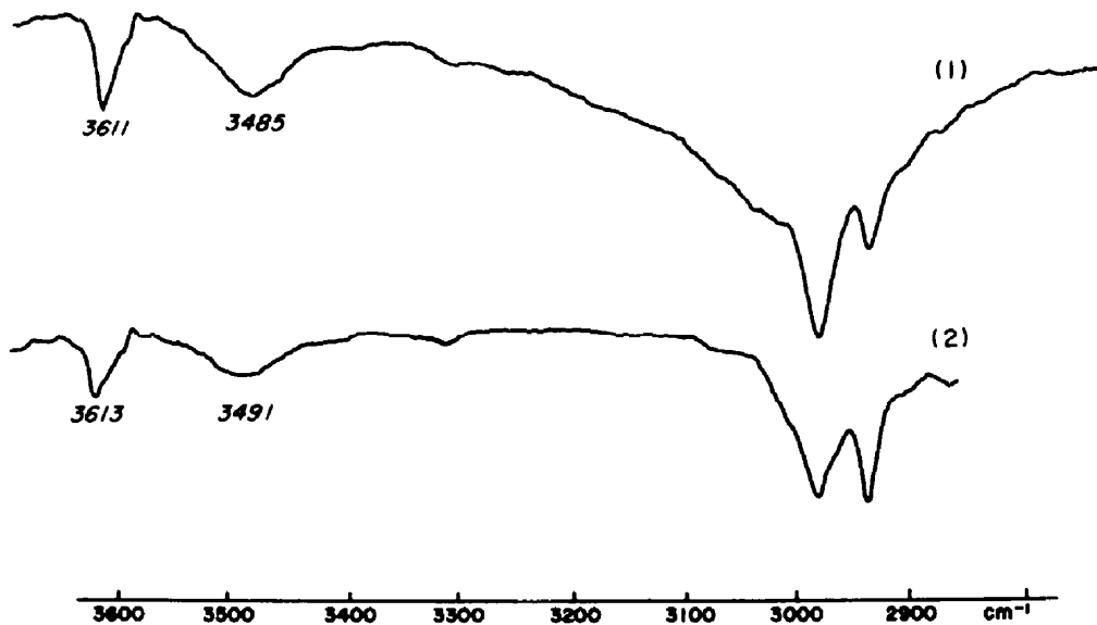
FIG. 5 IR spectra of IX (1) and X (2) in dilute CCl_4 .
